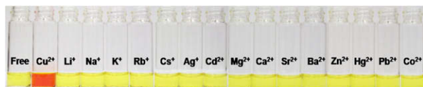
Figure 7. Visual color changes of 1 (50.0 \mu\text{M} ) upon addition of various metal ions in \text{CH}_3\text{CN} . From left to right: free 1 , \text{Cu}^{2+} , \text{Li}^+ , \text{Na}^+ , \text{K}^+ , \text{Rb}^+ , \text{Cs}^+ , \text{Ag}^+ , \text{Cd}^{2+} , \text{Mg}^{2+} , \text{Ca}^{2+} , \text{Sr}^{2+} , \text{Ba}^{2+} , \text{Zn}^{2+} , \text{Hg}^{2+} , \text{Pb}^{2+} , and \text{Co}^{2+} (250.0 equiv).
